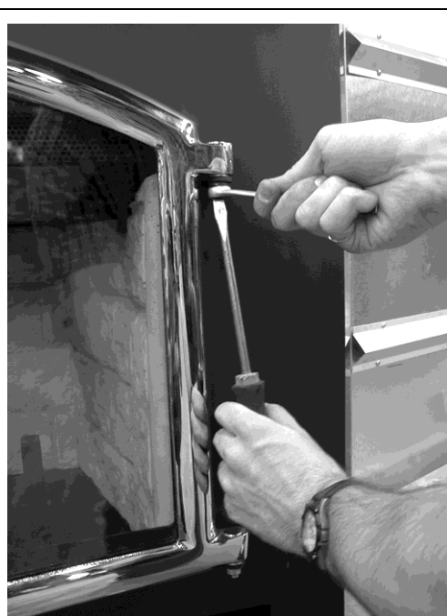
Figure 4 Door Hinge Adjustment
